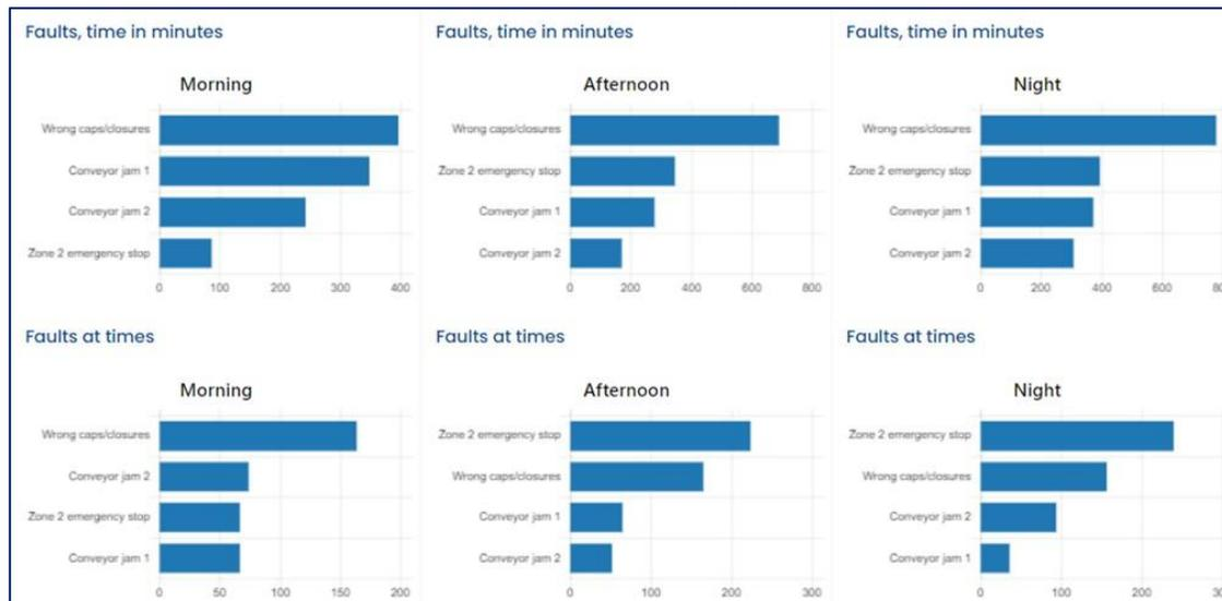
Here we find the last production data screen, where we can find the same graphs and data as the two previous screens, but in this case separated by work shifts.
